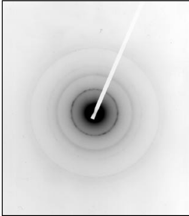
Figure 5.4: Diffraction pattern from the graphite area in Figure 5.1. This SAED was taken with a camera length of 1200 mm.
